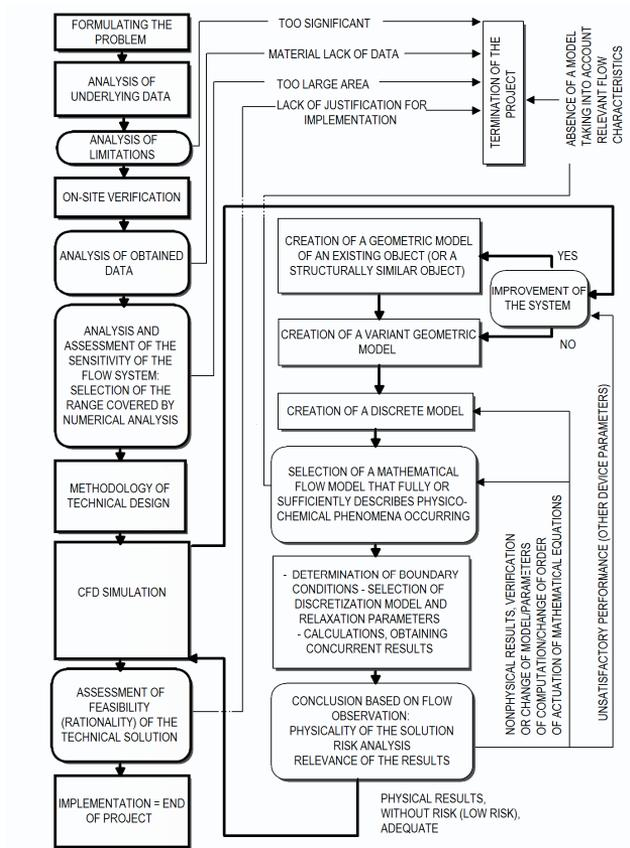
**Fig. 3.** Scheme for the design and modernisation of machines and flow-through systems using CFD software
