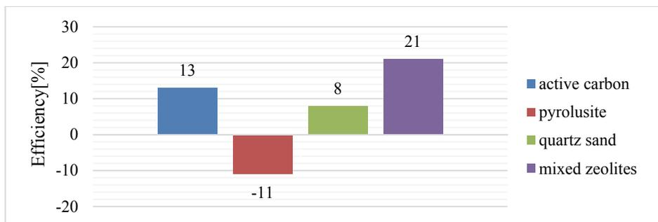
**Fig. 2.** Final efficiency of boron removal from the water through different filter bed materials
